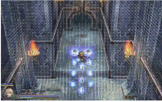
Fig. 6. A screen shot of Ys with its motion vectors overlaid. The motion vectors reveal how the macroblocks shifted since the last P- or I-frame in the recorded H.264 video. Because the avatar was moving downward, the motion vectors of the frame were generally pointing toward the top center on the screen.
